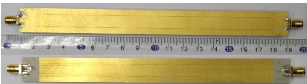
Fig. 5. The fabricated CRLH RSIW with 24 unit cells, acting as the feeding structure for the slot array antennas.
