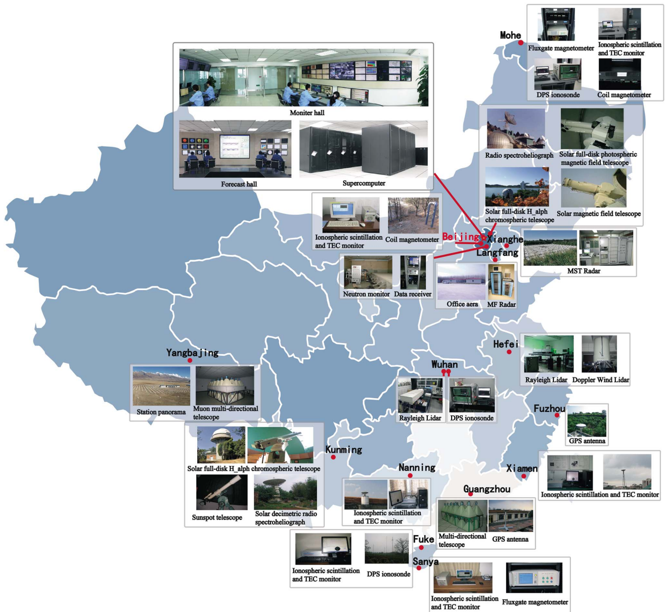
Figure 2. Distribution of observatories that form the Space Environment Monitoring Network (SEMnet) of CAS, along with the types of instruments deployed at each. There are three observatories in Beijing and one observatory in each other city. The central data center and operation center are at SEP/NSSC in Beijing.
