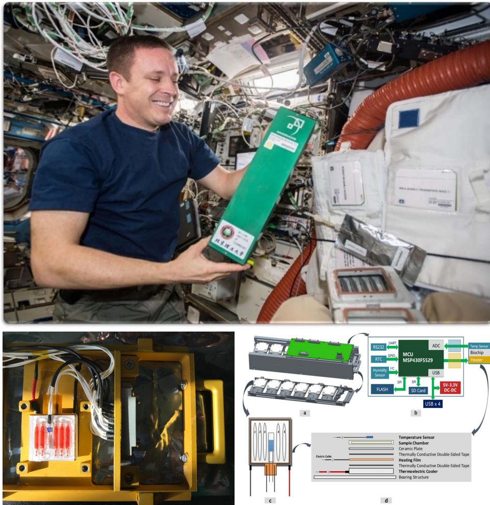
Fig. 5 Space molecular evolution payload and schematic schedule of space experiments in International Space Station
