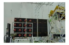
Fig.5 Deployment and illumination tests of the solar panels
