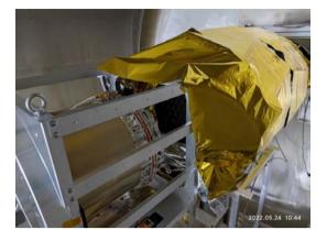
Fig.12 FXTOA-B (eROSITA FS) at IHEP 100 m X-ray facility
