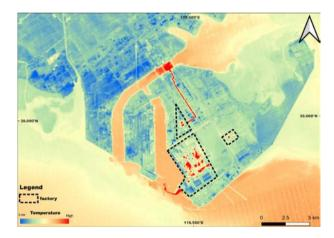
Fig. 3 SDGSAT-1 TIS Band 2 nighttime imagery showing coastal factories in Tangshan City, Hebei Province, China, on Jan. 10, 2024. Heat sources within the factory perimeters are visible in the imagery. Water bodies around factories also have an elevated temperature relative to their surrounding environments
