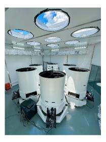
Fig.7 Array-type large aperture lidar
