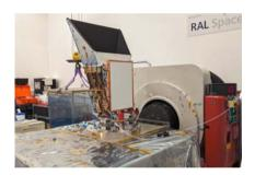
Fig.5 SXI Telescope PFM during Vibration Test Conducted at RAL Space (credit to S. Sembay, Leicester U., UK)
