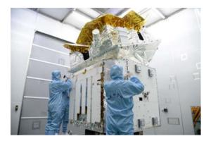
Fig. 6 EP satellite was being assembled within the specially-built EP clean chamber at the launch center in December 2023
