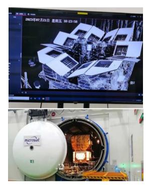
Fig.4 EP satellite flight model under thermal-balancing tests in Shanghai
