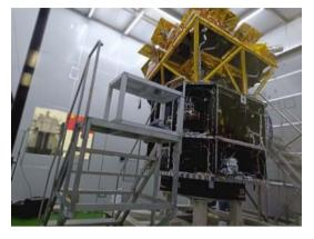
Fig.3 EP satellite integrated for end-to-end testing
