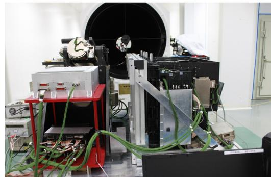
Fig.3 Joint test of satellite payload entanglement source
